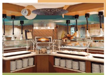
Highly styled, adjustable food shields by BSI, LLC, are incorporated into all the concepts, including the Pizza station, and enhance visibility to make the food the star. Designers spec'd adjustable shields to give foodservices the flexibility to switch a station to self-serve from full-service without a lot of effort, says Ron Lisberger, design project manager.
